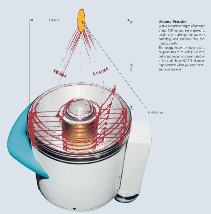
The cylindrical shock wave source is the most modern and efficient way of generating shock waves. A cylindrical coil covered with a copper membrane produces a cylindrical pressure wave. This wave travels outward and is then reflected by the parabolic reflector and thus focused precisely on the target. The cylindrical source is reliable and consistant and does not need any electrodes or acoustic lenses.
